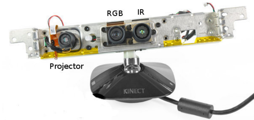
Figure 2.4: The internal structure of the sensor
